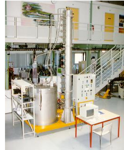
Fluidised bed reactor
